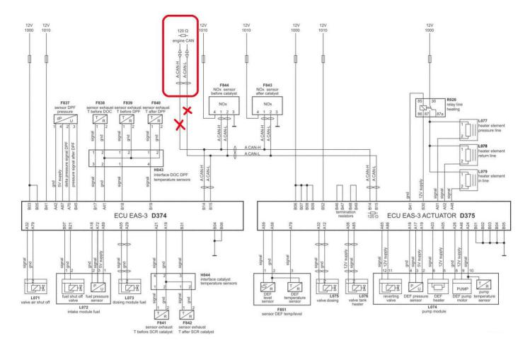
An EAS-3 system and its components are powered with the following fuses: D25(E444, 10A) and D26 (E443, 20A).
