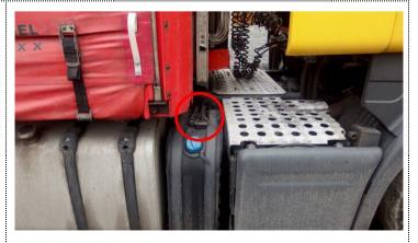
Disconnect the SCR plug, it has five pins. Two of five pins are gold plated, this is a CAN line. Now you need to connect the emulator wires to this plug (you can see the photos with connection scheme. If you have a new plug use it to solder emulator wires if you don't have a free plug so please use the one you have on the truck, cut the wires and connect the wires of the emulator.
