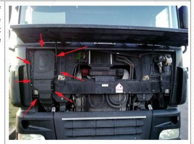
When you access the plastic box with all wiring you'll be able to connect emulator wires to necessary points. You need to find SCR system connector which has wires with numbers: 3781C (PIN 14 - red), 3780C (pin 13 - yellow), M34-2 (pin 19 - red), 1240A (pin 9 - red). Keep in mind that some trucks has wire 3781C named as 3781B and 3780C as 3780B.
