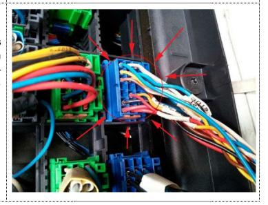
Now when you located all necessary wires you can connect emulator wires directly to the corresponding wires on the truck.
