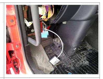
For the next step you need to remove fuse of SCR system. This is a F24-20A fuse, it is located in the fuse box (second fuse from the left in the second row), you can look for the fuse descriptions on the cover of the fuse box. You can find fuse box on the left side in front of passenger seat. Attention!!! On the Renault Magnum trucks you need to remove fuse F109 that is located behind the left side of the truck cabin near the battery. In ADR vehicles fuse layout may vary.
