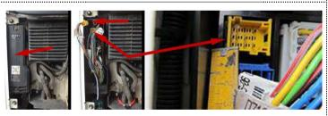
If you have ordered AdBlue Emulator V4 with the Volvo SCR plug just connect this plug to the socket instead of the yellow plug that you disconnected earlier. If you have ordered AdBlue Emulator V4 without a Volvo plug, you need to connect emulator wires to the original plug that you disconnected earlier. Look at the plug picture for more details where you need to connect emulator wires. When you connect the emulator wires to the plug connect it back to the socket.
