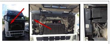
When you access the junction box take a look at the upper left corner of the box. You should see a yellow plug in the yellow socket, and this is what we are looking. It's a selective catalytic reduction system (SCR) plug. Remove this plug. Now connect the brown wire (ground) of the emulator to the truck (Important! Always connect ground wire first and disconnect last!). When the brown (ground) wire is connected, you can proceed to the next step.
