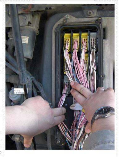
When all wires are connected, please turn on the ignition and start the engine. Make sure the indicator of AdBlue level shows half tank. If there are any faults at the time of switching off the engine, it is possible that after the AdBlue Emulator installation, the emission toxicity pictogram didn't go out on the instrumental panel. In this case, it is necessary to delete DTC fault codes from OBD and reset MIL parameter in the EDC tab. In these circumstances, MAN CATS is required.
